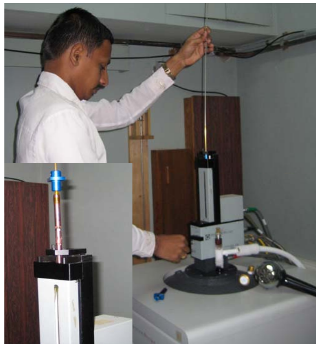
Figure 4: Mr Iyer loading the Mcell Ultra in a MPMS-XL7.
